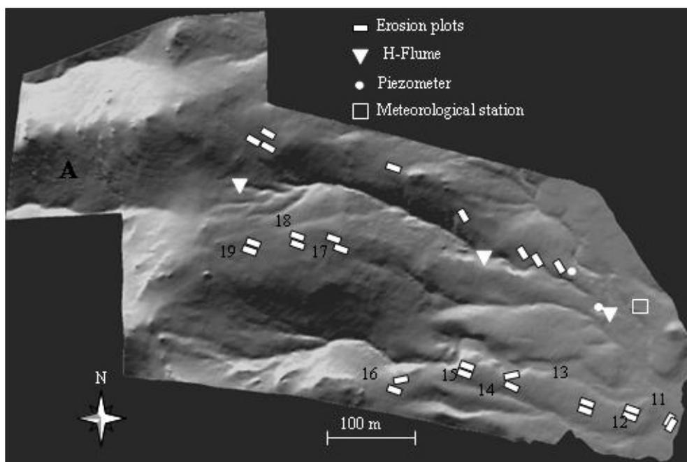
Fig 2.- Rambla Honda field site (map compiled from DEM at 1 m resolution), showing runoff-erosion plots, runoff gauges in the catchment and meteorological station.
