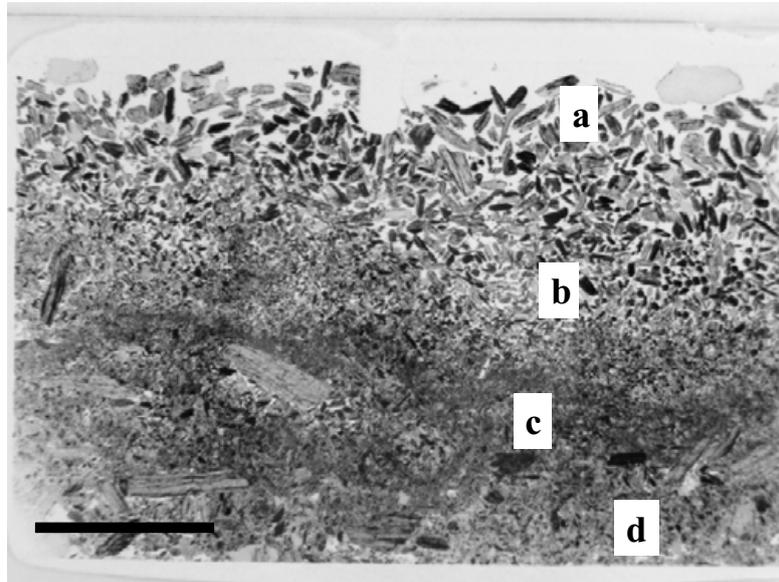
Fig 4.- Coarse pavement sieving crust. a = gravel and coarse sand layer, b = sand layer, c = very fine sand layer, d = heterogenous layer. Length of black bar = 15 mm.
